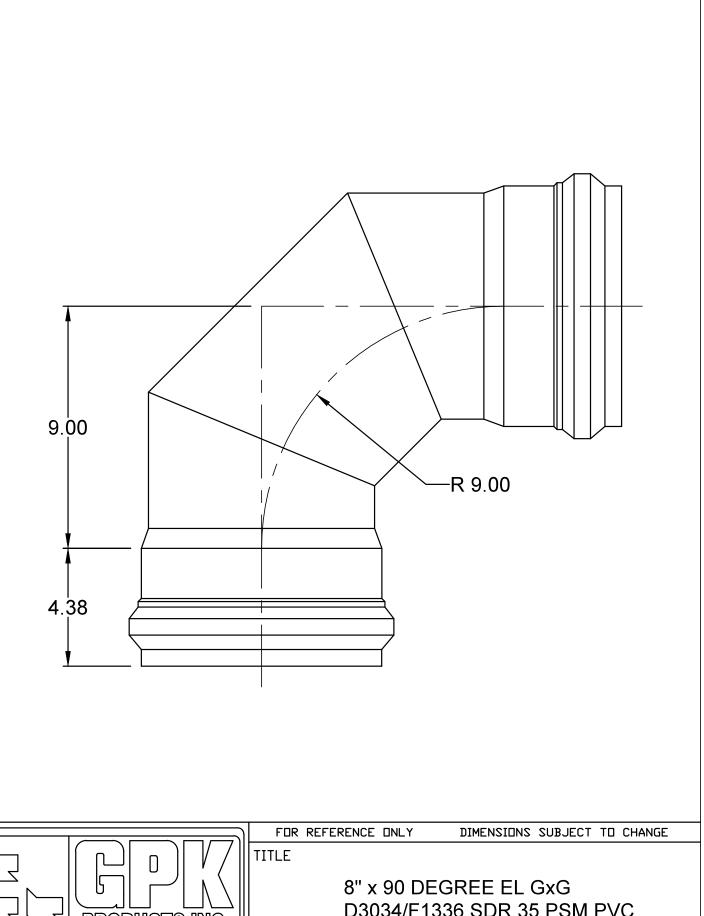
8" x 90 DEGREE EL GxG D3034/F1336 SDR 35 PSM PVC 1-800-437-4670 FARGO, ND DATE 10-13-11 SCALE NONE PART NO. 153-0008
